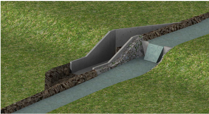
Step 2: Foundation, securing the walls
